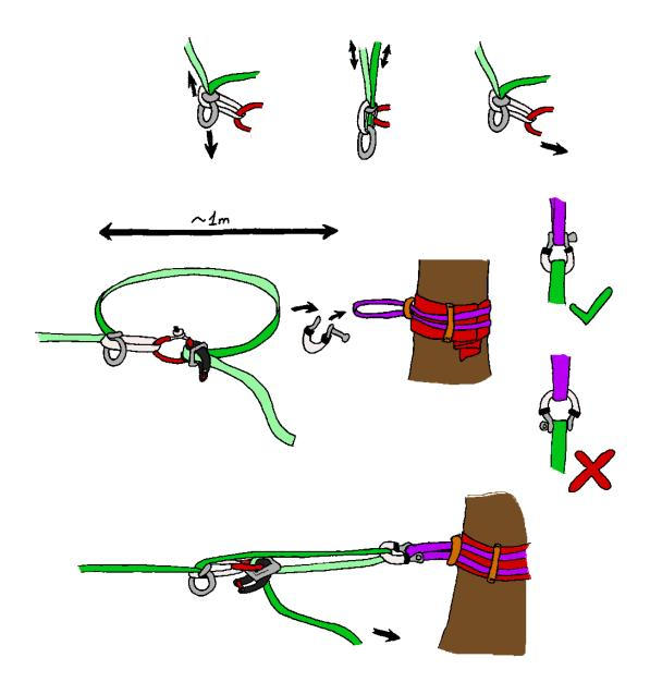
**Back-up** - Fit the end of the webbing through the ring, and then tie it back around the tree. This will prevent any slippage of the system, and provide extra safety.
