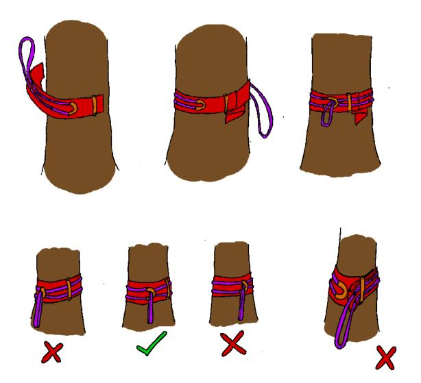
**Treesling -** Start by putting the padded loop on the side of one tree, facing towards the other tree. Wrap the Treesling around the tree, making sure that it stays flat to spread the pressure on the bark. Fold the excess padding, and fit the loop through the adjustment sling and the padded loop.
