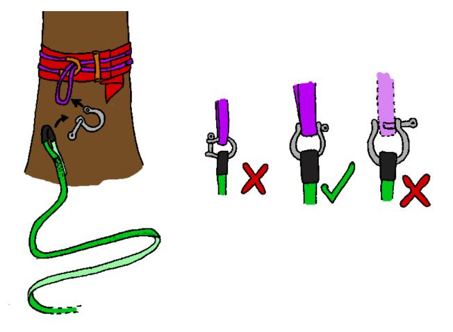
**Webbing-** Use the shackle without the low friction sleeve to connect the loop of the webbing to the Treesling. Make sure the shackle is properly closed and loaded in the main direction. Lay the webbing flat all the way to the other tree.
